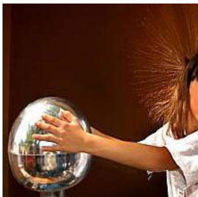
Photo: A classic demonstration of static electricity you may have seen in your school. When this girl touches the metal ball of a Van de Graaff static electricity generator, she receives a huge static electric charge and her hair literally stands on end! Each strand of hair gets the same static charge and like charges repel, so her hairs push away from one another. Photo courtesy of Sandia National Laboratories/US Department of Energy.
