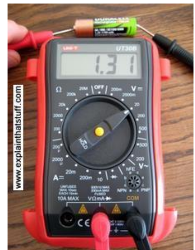
Photo: You can use a digital multimeter like this to measure voltage, current, and resistance.
