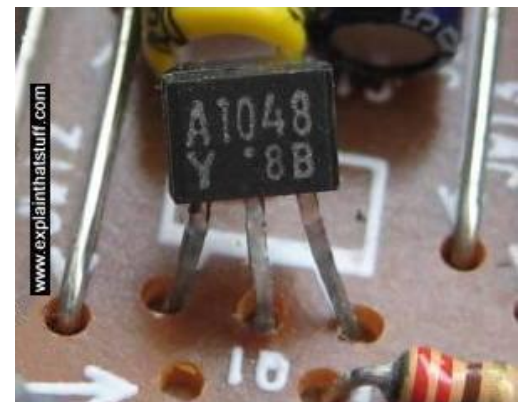
Photo: A transistor (a typical electronic component) on a circuit board. Components like this run on electricity, just like clothes washing machines, but they use much smaller currents and voltages.
