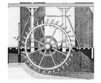
A very basic turbine (water wheel) using falling water to turn the shaft of an electric generator.
