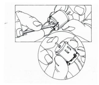
The motor cap should come off as shown. Next, separate the motor into three pieces by taking out the spinning coils.
