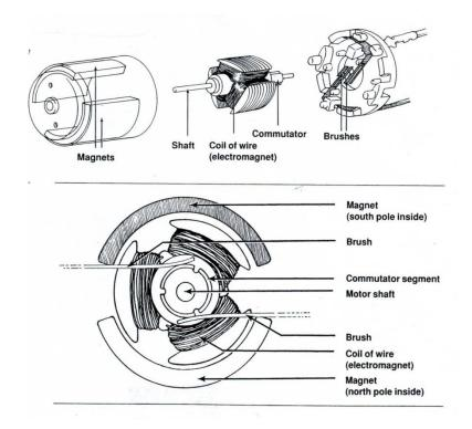
6. Look at all of the many parts that make up the motor. Think about the simple (spinning coil) motor you just built and compare it to this motor. Think about what the parts of each motor do. List pairs of parts that serve the same purpose. One part in the pair should be from the spinning coil motor you made and one part in the pair should be from this motor.
