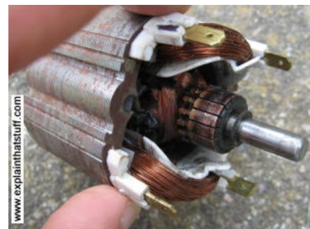
Photo: This is the motor from an old electric lawn mower. The copper-colored thing toward the front of the axle, with slits cut into it, is the commutator that keeps the motor spinning in the same direction.
