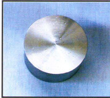
Figure 6. Pits are evidence of atomic motion in the aluminum base after numerous ball-plate collisions.
