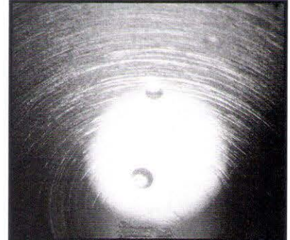
Figure 7. Several pits in the aluminum base are shown magnified 7.5 times.
