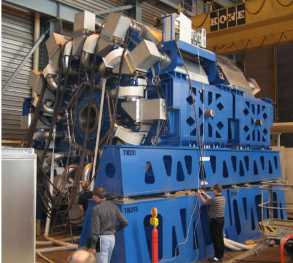
Figure 3: Direct drive neodymium-based permanent magnet generator for 3.5 MW wind turbine. Courtesy of The Switch (2008).
