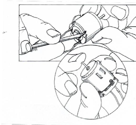
The motor cap should come off as shown. Next, separate the motor into three pieces by taking out the spinning coils.
