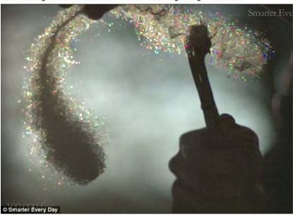
Fragile: Watching in slow motion, the tension pushing out from the middle shows the glass disintegrate into crystalline powder
