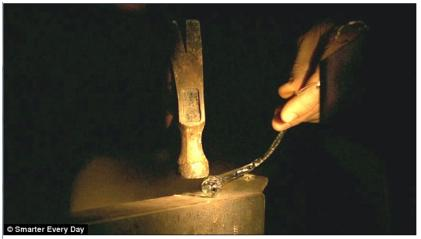
Tapering tail: While the front end is strong, the weak part of the teardrop shape is the thin end, which shatters the whole object quicker than the eye can see
